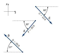
Note that when an angle above or below a horizontal is given, multiplying the magnitude by the cosine of the angle gives the horizontal component, and multiplying the magnitude by the sine of the angle gives the vertical component.
